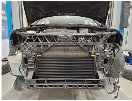
Loosely install the brackets to the intercooler with the included M6x12 4mm allen screws then lift it in place so that the radiator stands in the radiator seats in the intercooler and secure it to the AC condenser and radiator with the two T30 screws removed in previous step. Before tightening all 4 screws, make sure there is space between the intercooler and the AC-condenser.
