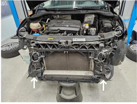
Remove the temp sensor from the radiator support. Support the radiator support and remove 6x 13mm hex screws (three on each side) then remove the bumper beam.
