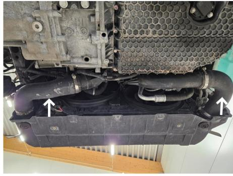
Remove the 2x T20 screws holding the airduct (marked with arrows in picture) and remove it from the car. Then disconnect the hood latch sensor.
