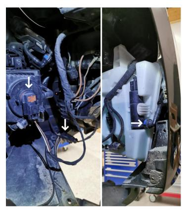
Remove the fog light electrical connectors on both sides and the bumper harness connectors on the left. Then disconnect the washer fluid line from the pump on the right side (use a clean bucket to catch the fluid that comes out from pump and lines so you can re-use it).
