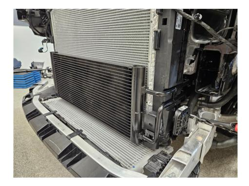
Install the do88 transmission cooler. Pull of the caps and attach the oil lines quickly to prevent leakage. Make sure the green clips have locked correctly onto the connections.
