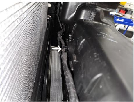
Unclip the wiring harness shows on the photos. Also disconnect cable connectors for the radar unit, temperature sensor (upper grille air guide), 2x horns, 2x airbag sensor (each end of the bumper bar).
