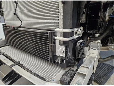
Remove the bumper bar. You will need to pry the marked brackets outwards to let the guide pin pass underneath it.
