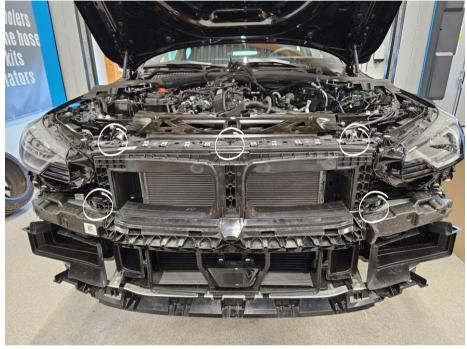
Remove 10x Torx T30 screws from the top of the bumper. Then remove the bumper.
