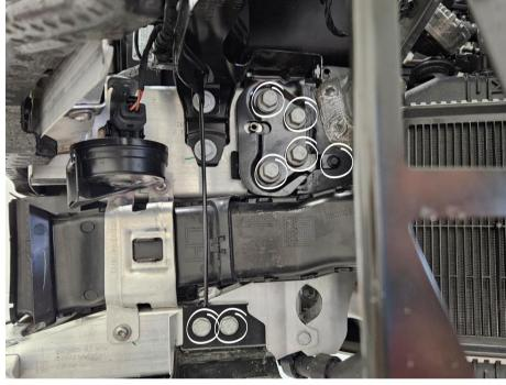
Remove 1x Hex 10mm and 2x Hex 13mm hex screws from the auxiliary radiator on the left side. Lean it backwards and lift it to the side and secure it to the vehicle with a zip tie. Also remove the plastic air guide.
