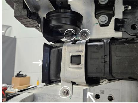
Remove 3x Hex 13mm screws, one of the is located on the backside where the arrow is showing.
