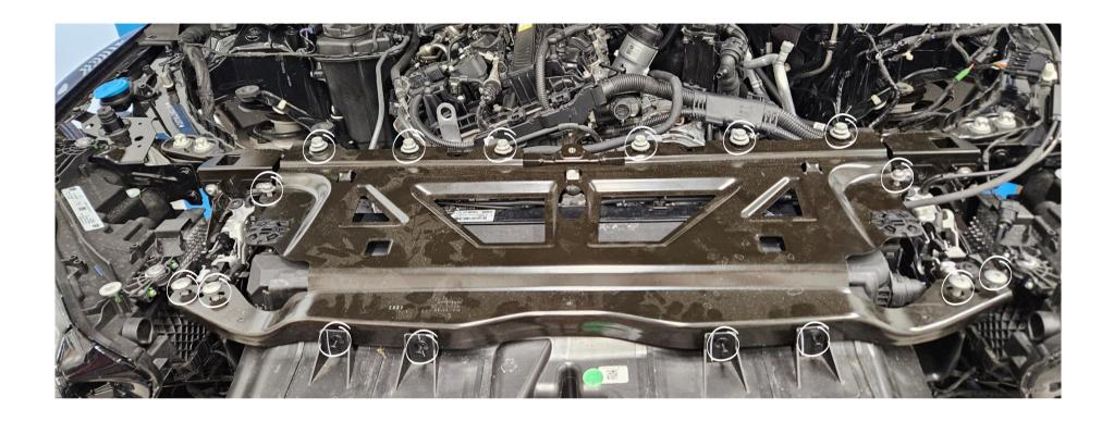
Remove 4x Torx T40 screws / 2x T30 screws / 6x Hex 13mm screws / 4x plastic clips. Then remove the large bracket on top of the radiator.
