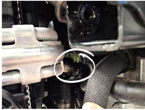
Pre-fill the do88 transmission cooler (use oil according to manufacturer specifications). Then cap the connections with the included caps to prevent oil leakage during installation.
