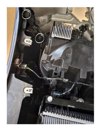
Remove 2x Hex 8mm screw securing the bumper in the upper corner of the wheel arches on both sides.
