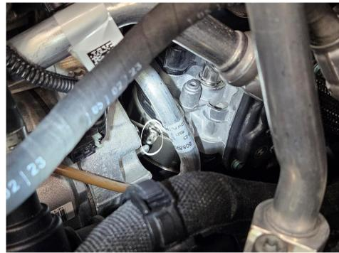
Remove the 4x 10mm Hex screws (arrows) holding the y-pipe to the engine. Two on the top and two on the bottom (there is standoff screws between y-pipe and engine that may loosen from engine when removing the 10mm hex screw). When the y-pipe is loose remove the turbo side hoses by undoing the 4 c-clips, two on the y-pipe, one on the front turbo and one on the pipe from the rear turbo. Remove the y-pipe from the car.
