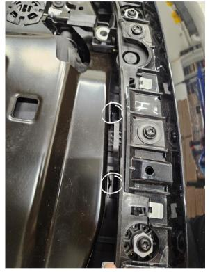
Remove 6x 13mm Hex screws (upper arrows) and 7x Torx T30 screws (Circled) then pull the upper part of the bumper cover forward to reveal and remove all 4x Torx T40 screws (lower arrows). Loosen the hood cable from the 3 tabs.
