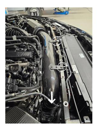
Remove the two plastic clips holding the intake pipe to the radiator support bar and undo the C-clip or hose clamp holding the intake pipe to the front turbo inlet. Then remove the left intake assembly.
