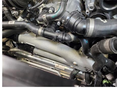
Install the long silicone hose between the upper inlet of the y-pipe and the charge pipe coming from the rear turbo.
