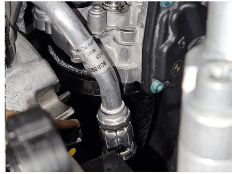
From the front turbo outlet hose, transfer the OE sealing ring and C-clip to the do88 Performance turbo adapter.
