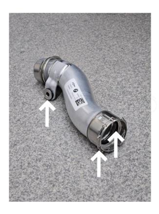
Transfer the OE sealing ring, C-clips and bushing with sleeve to the do88 Performance charge pipe.
