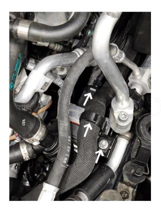
Remove the 10mm Hex nut and release the clip holding the radiator hose on top of the auxiliary water pump located on the chassis beam on the left side of the engine. Disconnect the electrical connector from the water pump and move the water pump to the side.
