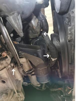
Loosen the hose clamps on the intercooler inlet and outlet hoses, then remove them.
